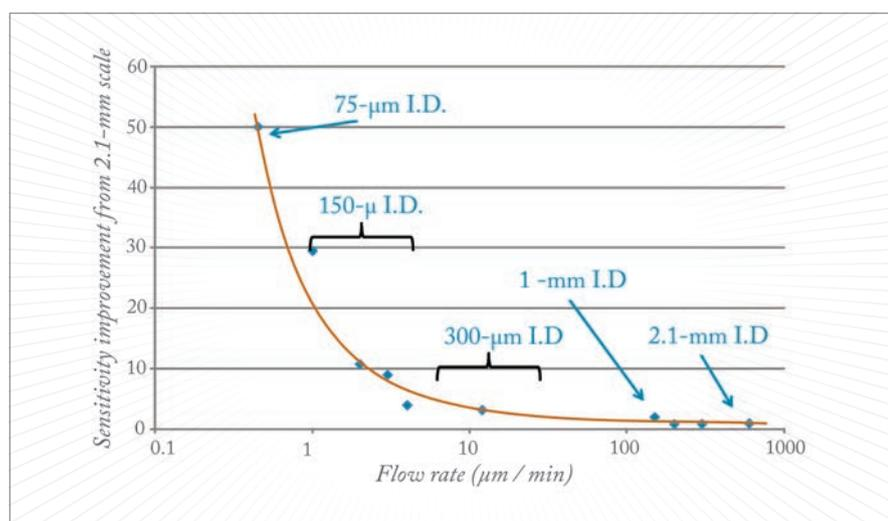
Figure 2. The average signal enhancement with reducing column diameters and flow rates in comparison to a 2.1 mm format for a series of small molecules (lidocaine, propranolol, dextromethorphan, fluconazole, alprazolam, and verapamil). All injections were made with the same concentration solution and a volume of 1 microliter.
